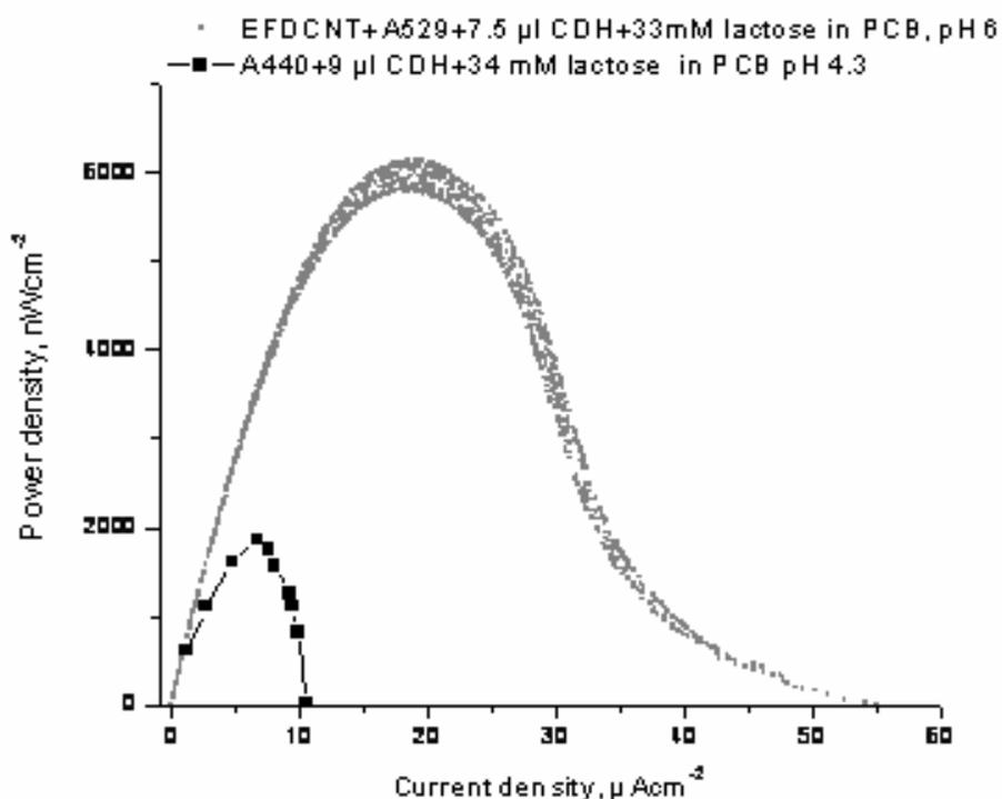
**Figure 3.** Dependence of the power density on cell voltage (left) and on current density (right) for a BFC assembled from cellobiose dehydrogenase/Os redox polymers bioanode and laccase/Os redox polymer biocathode. The redox polymers used for entrapment of CDH were with formal potentials respectively ca. +200 mV (1) and -50 mV vs Ag/AgCl (2).
