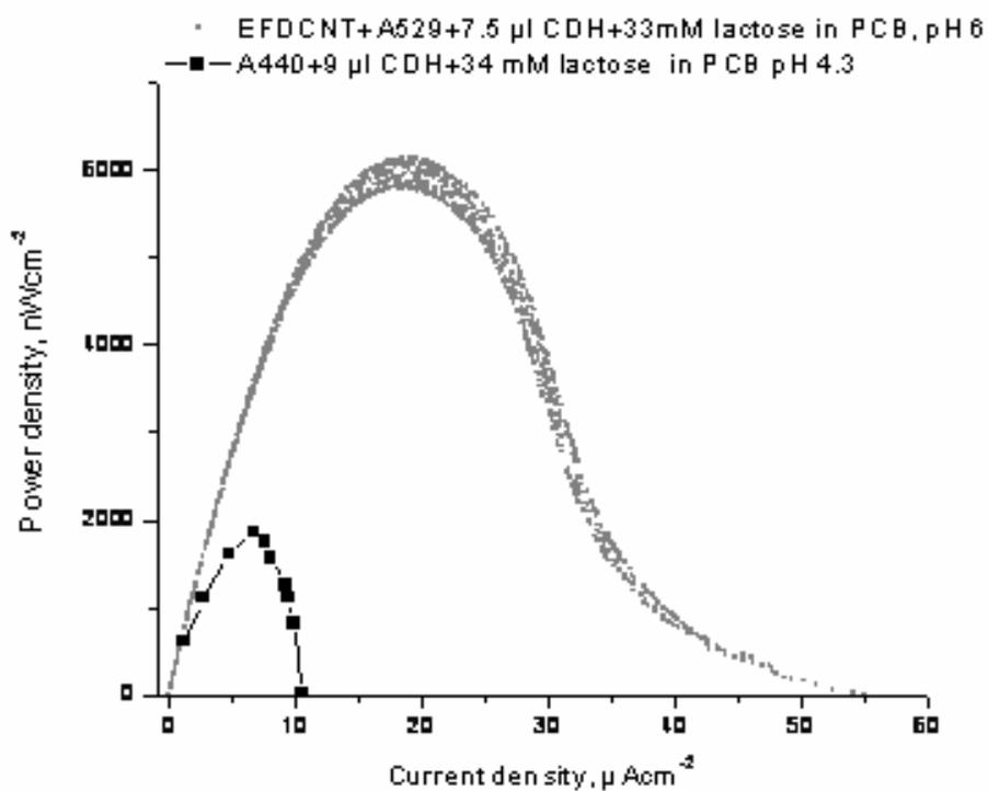
**Figure 3.** Dependence of the power density on cell voltage (left) and on current density (right) for a BFC assembled from cellobiose dehydrogenase/Os redox polymers bioanode and laccase/Os redox polymer biocathode. The redox polymers used for entrapment of CDH were with formal potentials respectively ca. +200 mV (1) and -50 mV vs Ag/AgCl (2).
