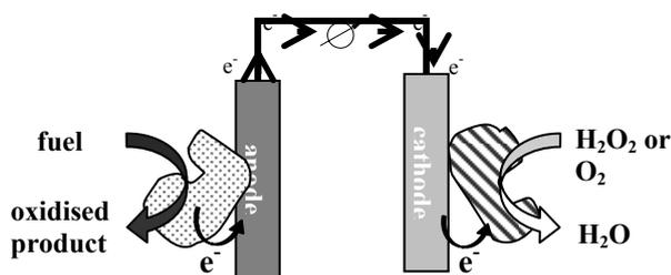
**Figure 1.** Scheme of a membrane-less biofuel cell.
