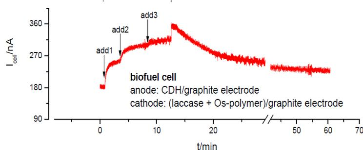
**Figure 2.** Current output (original record) of a BFC assembled from adsorbed CDH- bioanode and laccase trapped in Os-redox polymer biocathode, pH 4.3.
