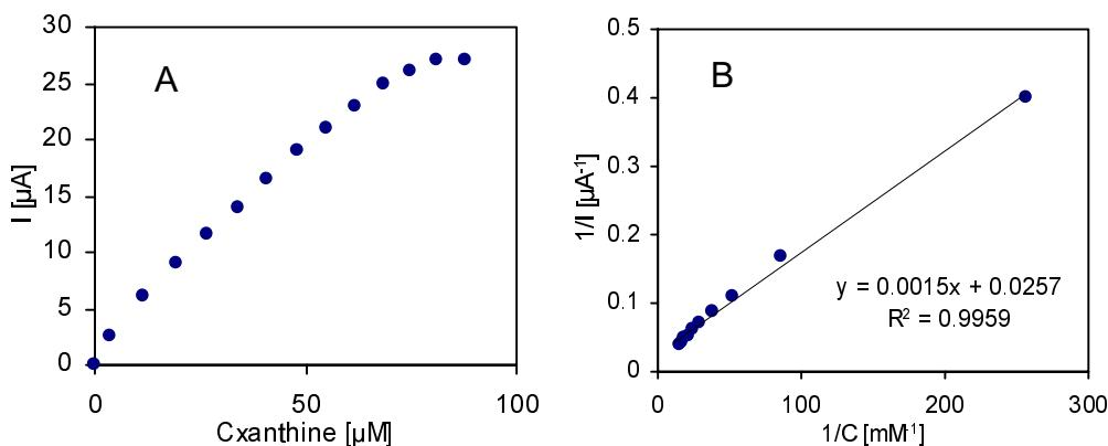
**Figure 2.** A - Steady-state response of the enzyme electrode type B as a function of xanthine concentration; B – Lineweaver – Burke plot. Applied potential -50mV(vs. Ag/AgCl); background electrolyte: 0.1 M phosphate buffer, pH=8.4; temperature 25 °C
