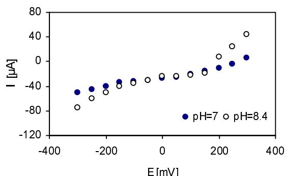
**Figure 1.** Polarization curves of graphite modified electrode Pt:Pd(30:70)/Cgmz in 0.1 mM  $\text{H}_2\text{O}_2$ , background electrolyte: phosphate buffer; reference electrode Ag/AgCl; temperature 20°C
